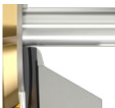
Small axial relief: stronger tool Large axial relief: weaker tool
